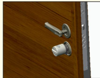
Tighten the 4 fixing screws.
